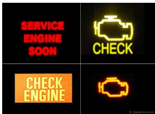
Figure 3. MIL and CHECK ENGINE light combinations [18]
