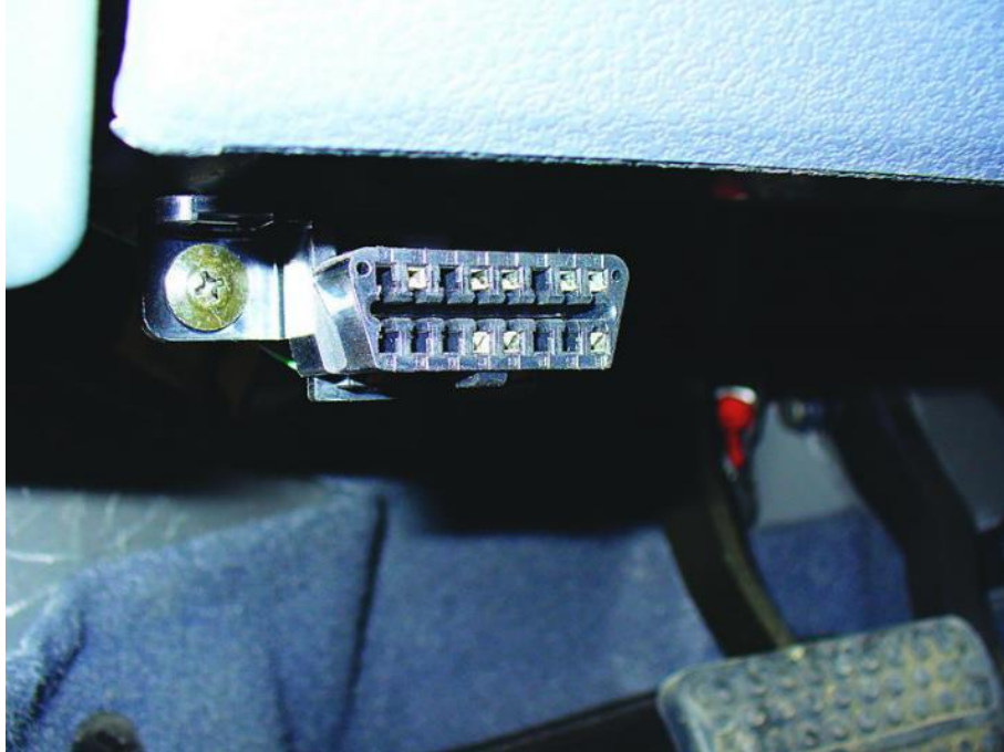
Figure 5. OBD socket under the dashboard [20]
